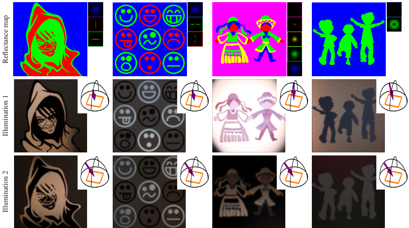
Figure 11: Fabricated patterns viewed under white illumination at varying directions. First row: Design mask and the reflectance types involved (synthetic). Second and third rows: images of pattern under two different lighting directions (real). See supplementary video.
